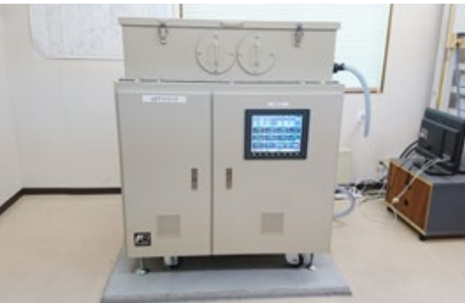
Continuous measurement system for radioactivity concentration in dust
